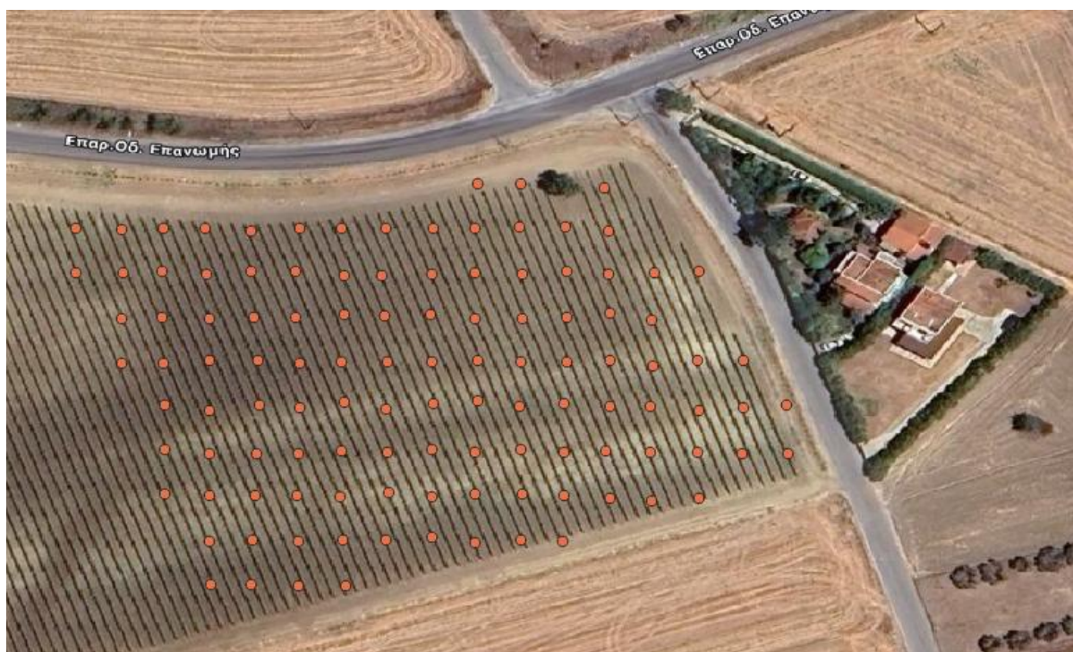
Figure 20. Distribution of PSR+3500 field spectra acquisition points across the vineyard. Sampling locations correspond to Sentinel-2 pixel centers and were complemented by soil sample collection for subsequent laboratory analysis.
