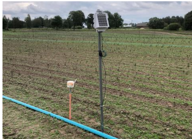
Figure 32: Node with soil moisture and temperature sensors in peppermint field in Latvia
