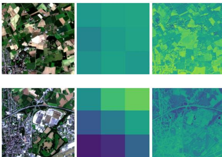
Figure 26. Top to bottom: Sentinel 2 super-resolved RGB image, Sentinel-3 SLSTR thermal image at 1km resolution, Thermal sharpened image at 10 m resolution.
