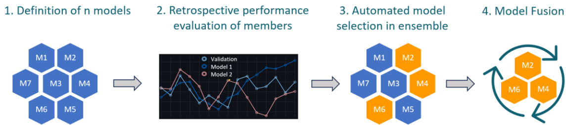
Figure 27: Methodology of the time series forecasting framework building ensemble models from best performing members by time lagged validation.
