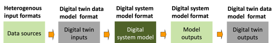
Figure 1. Digital twin data model usage between heterogenous data source inputs, digital system model and digital twin output.
