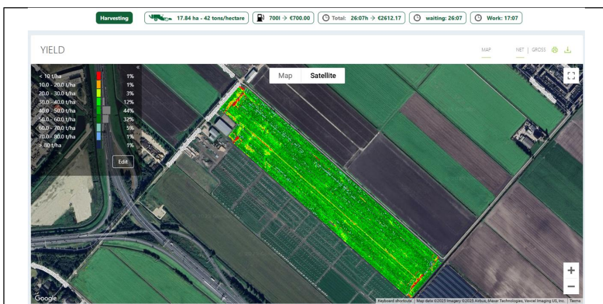
Figure 2. Yield (tons/ha) measured on the field by an AVR potato harvester equipped with a yield measurement system. Lower than average yields are shown in red, average yields in green, higher than average yields in blue.
