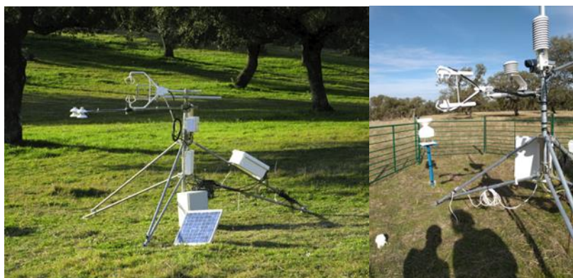
Figure 24: Sensors installed in grasslands in the Pedroches area
