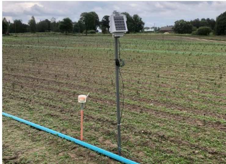
Figure 3: Node with soil moisture and temperature sensors in peppermint field in Latvia
